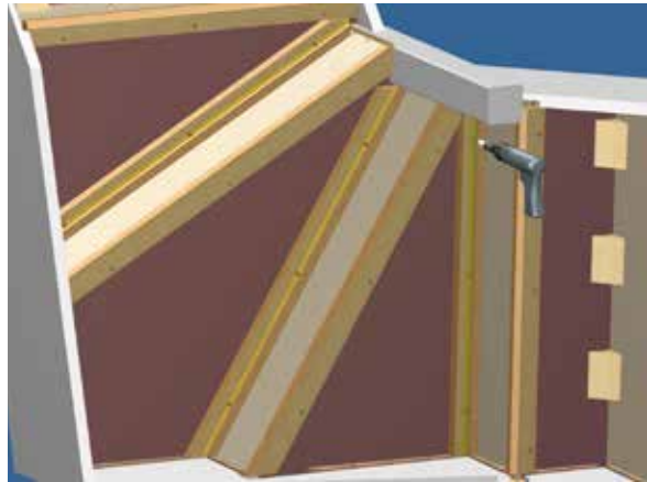
2. Screw the batten to the tread and riser intersection.
