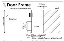
The frame to wall gap must be filled with stone wool or sealed with intumescent mastic if less than 6mm wide.
