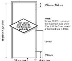
Measure from the top of the floor covering to the underside of the door.
