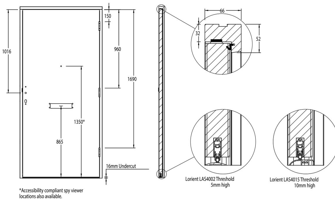
Dimensions shown on drawing detail the default hardware locations, based on standard sized flush doors. Dimensions will vary slight on Made to Measure products and moulded options to suit the design of the doorset.
