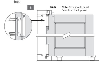
Adjust the top and bottom pivot hinges to ensure the door is vertical and set 5mm from the top track.
